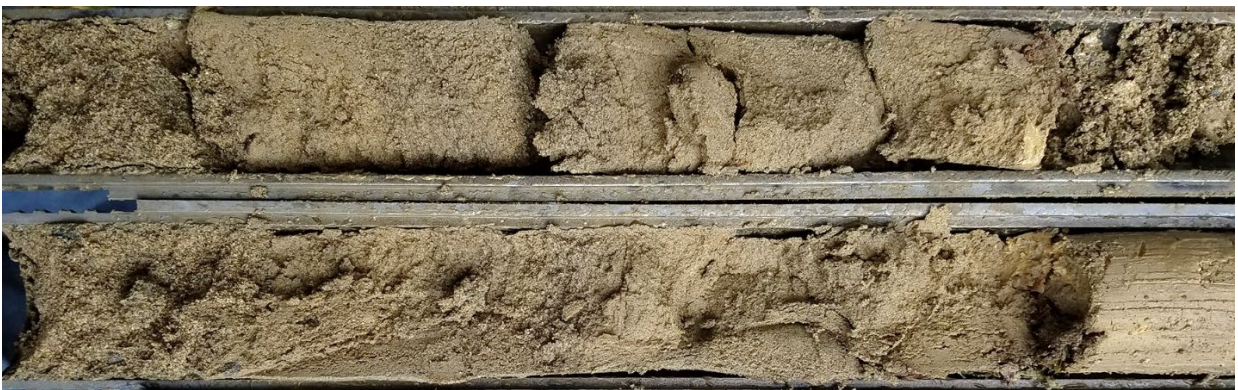
Plate 4 –Qvlc | Medium dense SILT | PG-3, S-1 @ 5-6½ feet.
